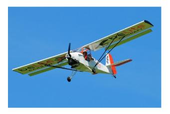
Belite Aircraft has solved this problem and offers an ultralight with the feel of a real airplane. The Belite incorporates stronger, lighter carbon fiber technologies, instead of older steel, wood, or aluminum. The result is a full-featured airplane with a real instrument panel that meets the 254 pound limit specified in FAR Part 103.
