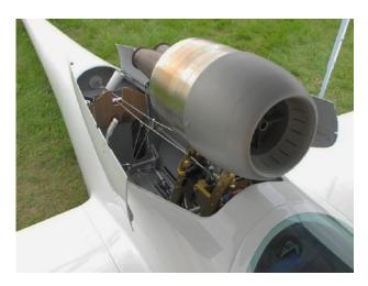
The PBS TJ-100 weighs only 45 pounds and produces 240 pounds of thrust. Desert Aerospace has modified the two-seat TST-14J sailplane to accept the tiny jet engine. For takeoff, the jet engine sits directly behind the cockpit and allows the glider to climb at more than 900 feet per minute.
