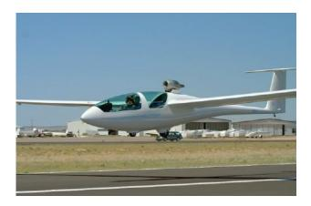
Several people have experimented with jet engines on sailplane, but a small New Mexico company plans to start selling them soon. Desert Aerospace is building an alternative to the expensive self-launch gliders made in Germany by combing a high-performance glider and a jet engine designed for use in unmanned aerial vehicles, both made in the Czech Republic.
